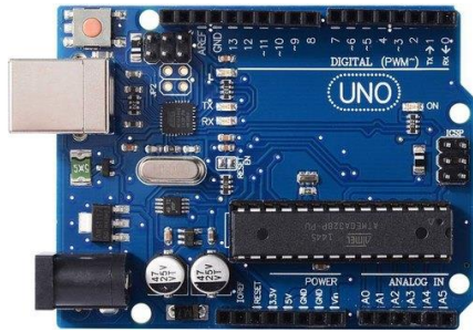
Figure 2: Arduino Uno R3
